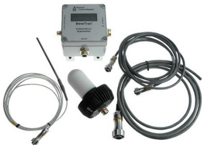
The Dewtran uses chilled mirror technology.
