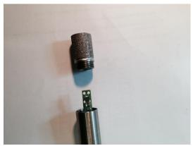
2: Gripping the sides of the exposed tip board with two fingers (see arrows below) gently pull up disconnecting the tip board from the internal main board.
