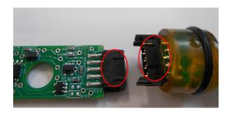
4:When the grooves align gently push down on the top of the tip board until you hear or feel a click.
