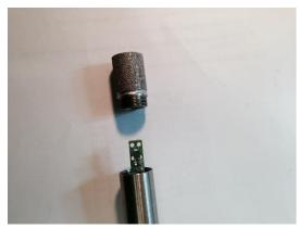
2: Gripping the sides of the exposed tip board with two fingers (see arrows below) gently pull up disconnecting the tip board from the internal main board.
